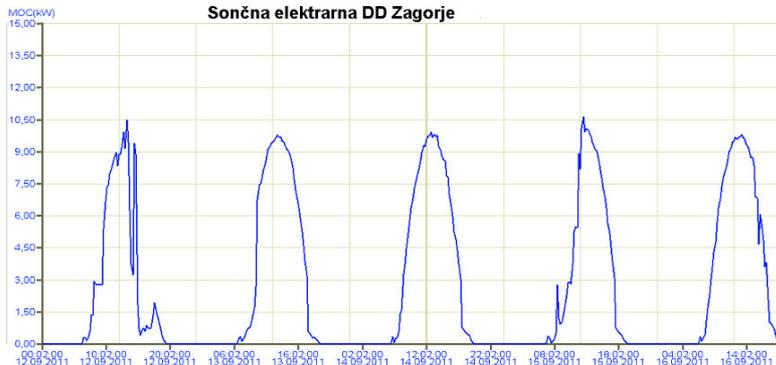
Fig. 12. Measurements of electricity production with 2 min sampling rate from PV plant *Delavski dom* monitoring system for same period as Figure 9.
