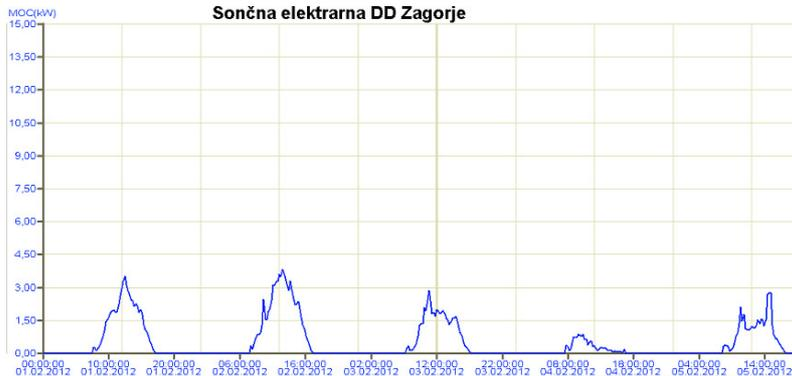
Fig. 14. Measurements of electricity production with 2 min sampling rate from grid connected PV plant
